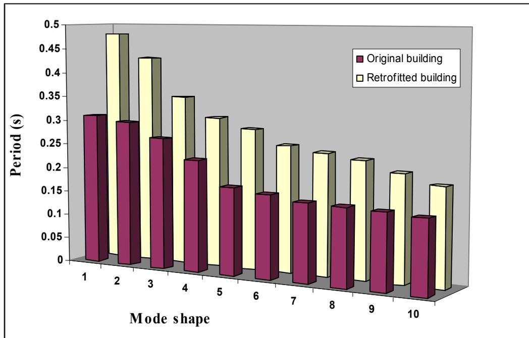
Fig. 10. Comparison of the mode shapes period for original building and retrofitted one
