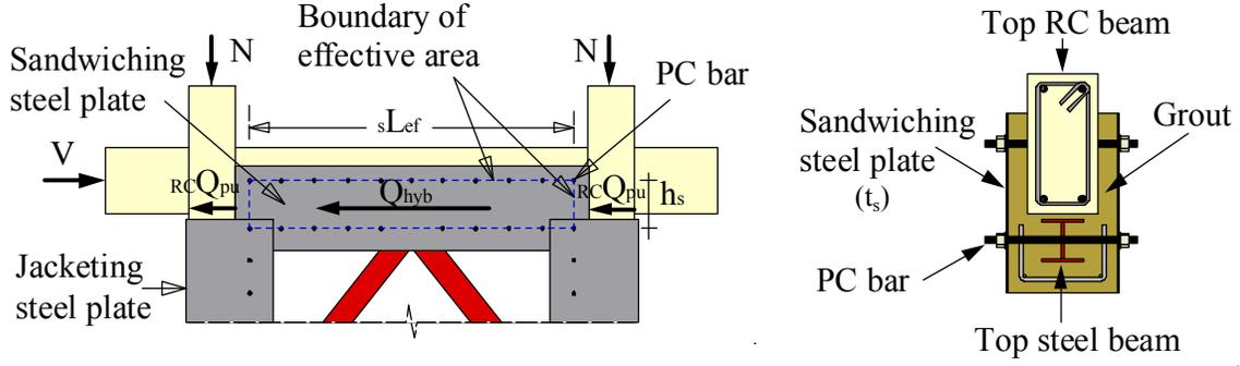
Figure 10. The geometry details of the hybrid connection
