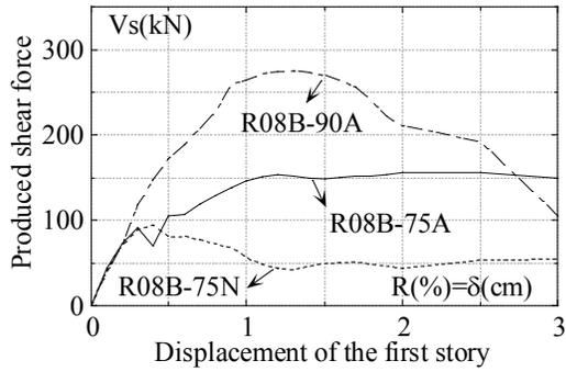
Figure 7. Shear force of one steel plate at the top connection
