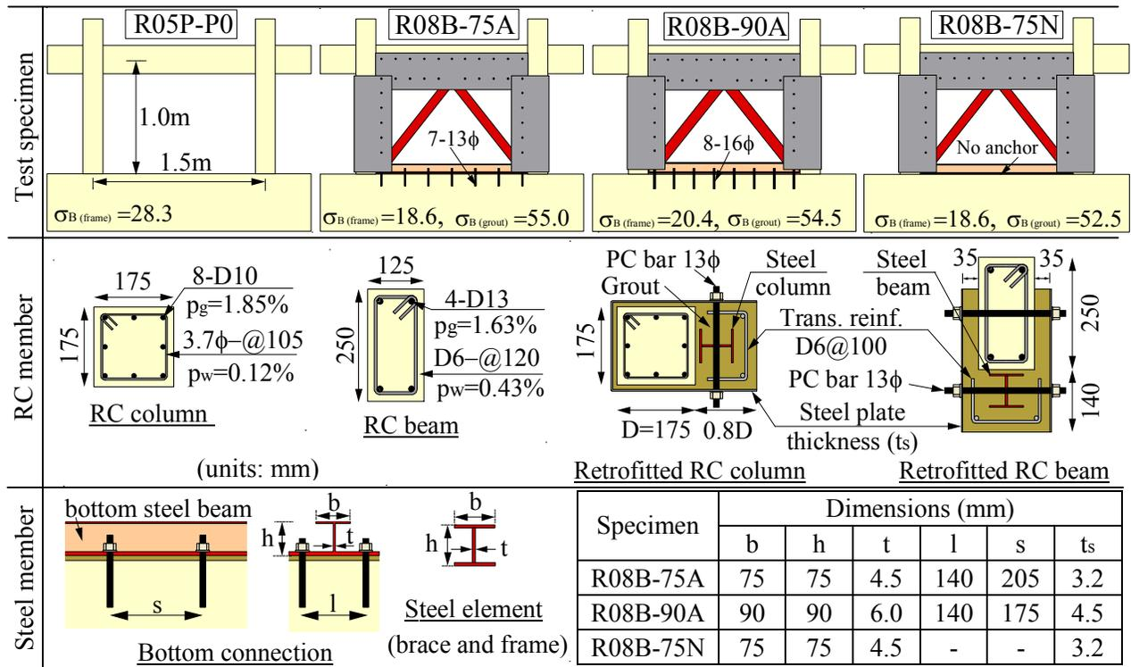
Figure 2. Details of the test specimens
