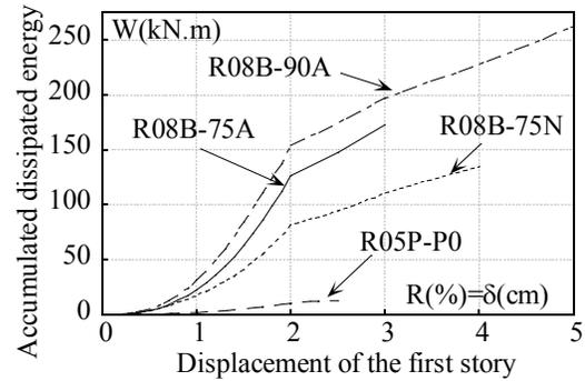
Figure 8. Accumulated dissipated energy of the test specimens
