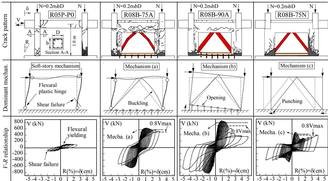
Figure 6. Experimentally obtained results of the test specimens
