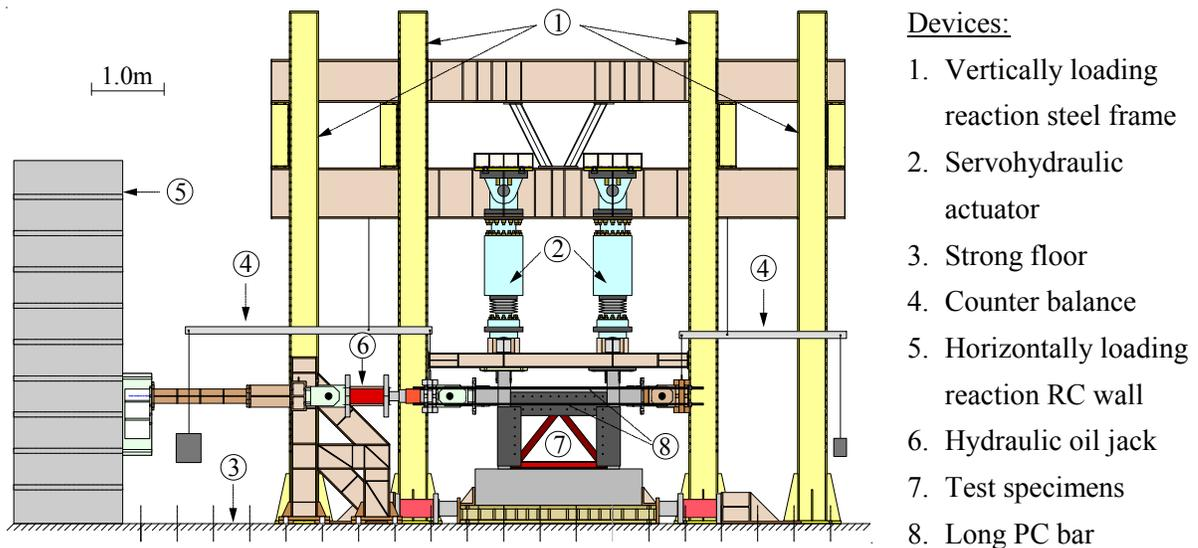
Figure 5. Test setup
