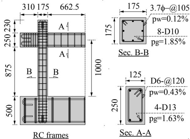
Figure 3. Reinforcement details
