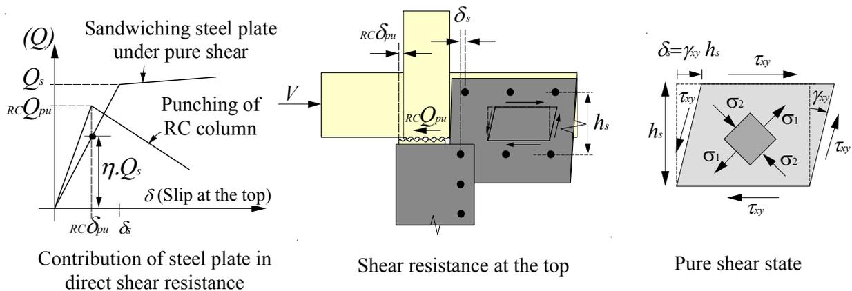
Figure 9. Contribution of sandwiching steel plate in direct-shear resistance
