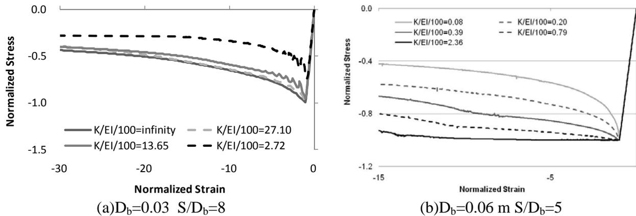
Figure 6. Spring stiffness effects on average stress strain curves
