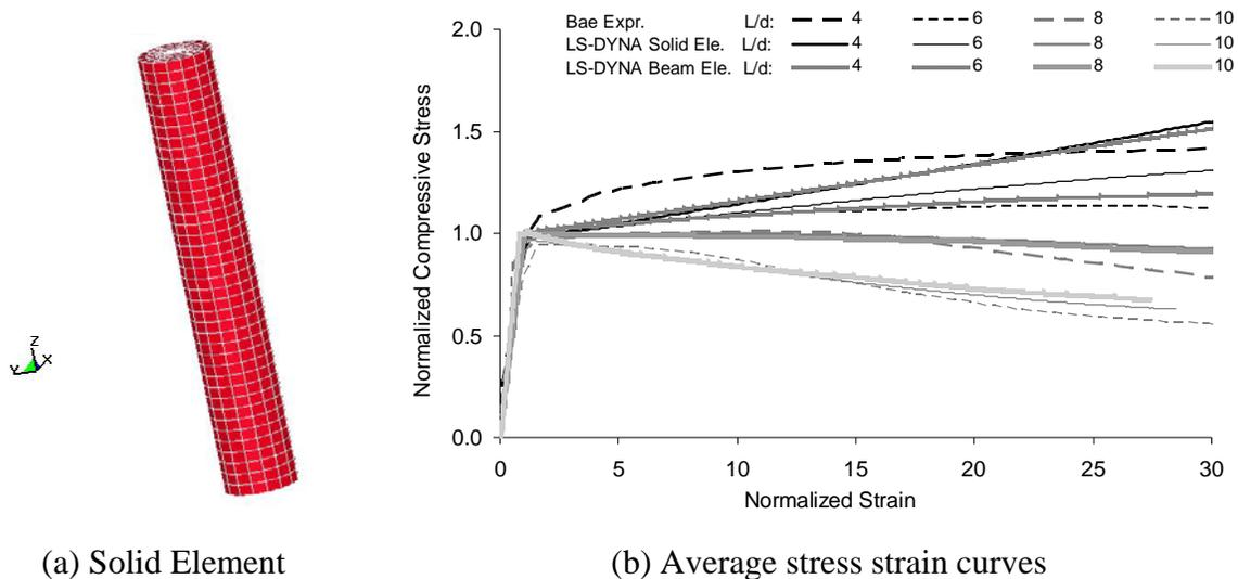
Figure 1. Single bar model in LS-DYNA
