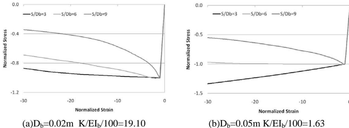
Figure 7. Hoop spacing and bar diameter ratio effects on average stress strain curves
