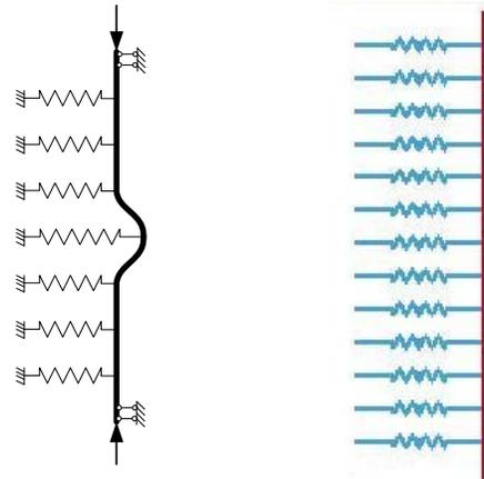
(a) Schematic diagram (b) LS-DYNA model
