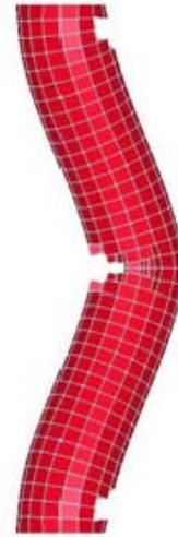
Figure 3. Negative volume cause deletion of elements
