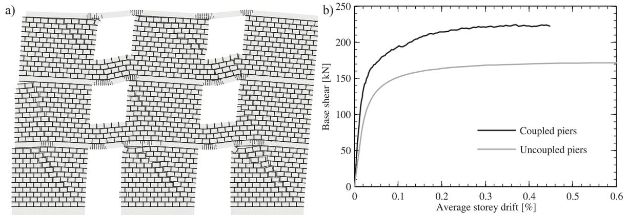
Figure 2. Deformed shape of the URM wall at an average storey drift of  $\delta=0.4\%$  (a, displacements are magnified by a factor of 20) and pushover curve of the URM wall in comparison to the pushover curve of uncoupled piers (b).
