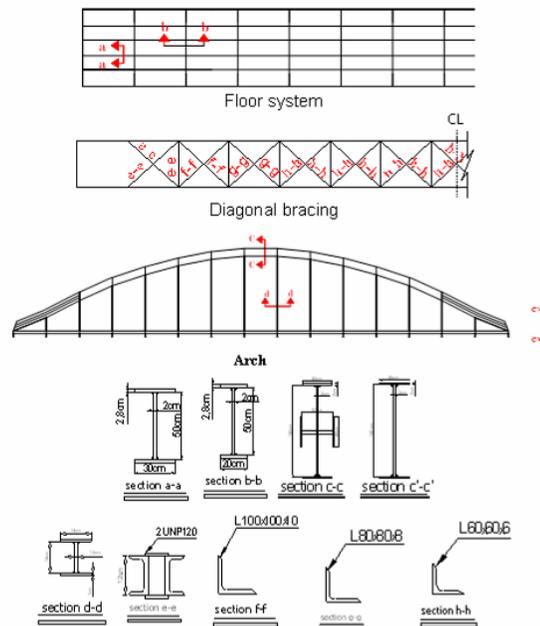
Figure 3. Geometry of the bridge
