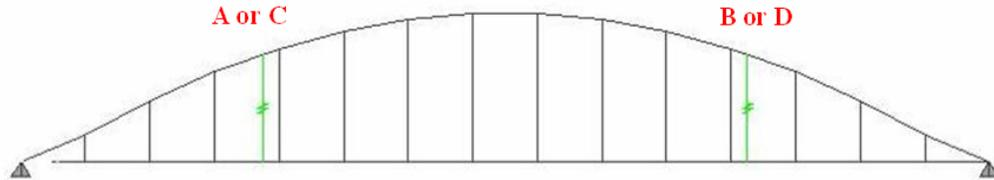
Figure 8. Placement of TMDs at quarter points
