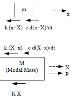
Figure 2. Free-body Diagram of the TMD and Structure
