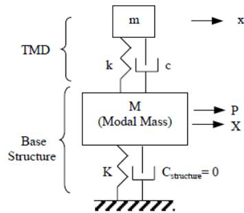
Figure 1. Operating Principle of a TMD
