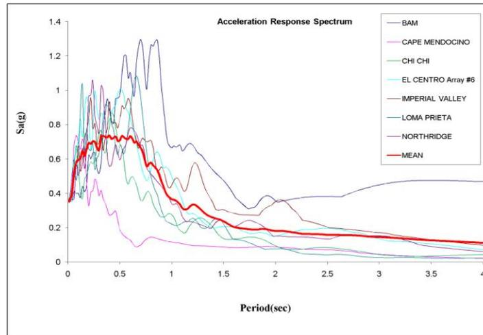
Figure 6. Acceleration response spectrum of selected ground motions
