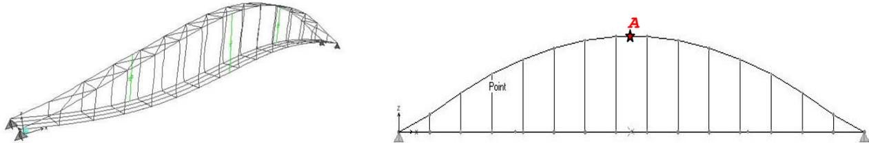
Figure 10. Placement of TMD at the quarter points of one arch and at the middle of the other arch
