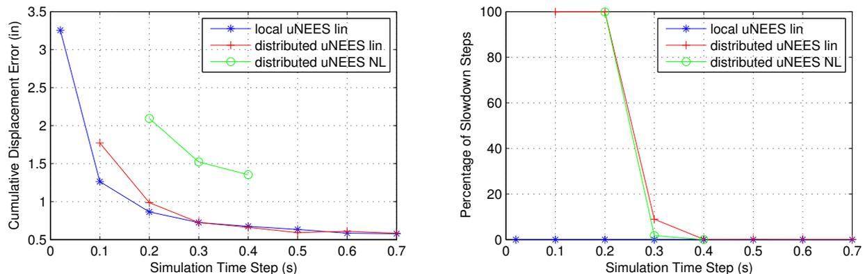
Figure 5. (a) Cumulative displacement error (b) Percentage of actuator slowdown steps.
