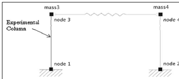
Figure 1. One Bay Frame Model Geometry.
