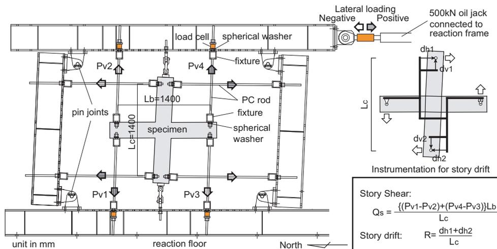
Figure 5. Loading set up and instrumentation for story drift
