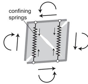
Figure 1. Deformation and moment resisting mechanism in a beam-column joint
