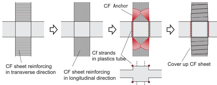
Figure 2. CFRP layout and procedure for retrofitting of beam-column joint
