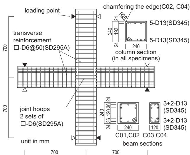
Figure 3. Geometry and reinforcing detail of the specimens
