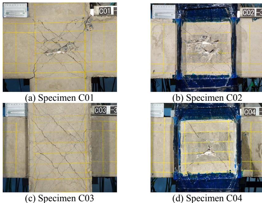
Photo 1. Failure pattern of the specimens at the cycle of 3% story drift ratio
