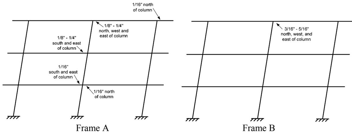
Figure 8. Vertical slab separations in north loading of Cycle 4.
