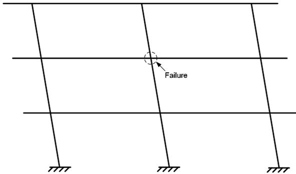
Figure 6. Frame B failure location.
