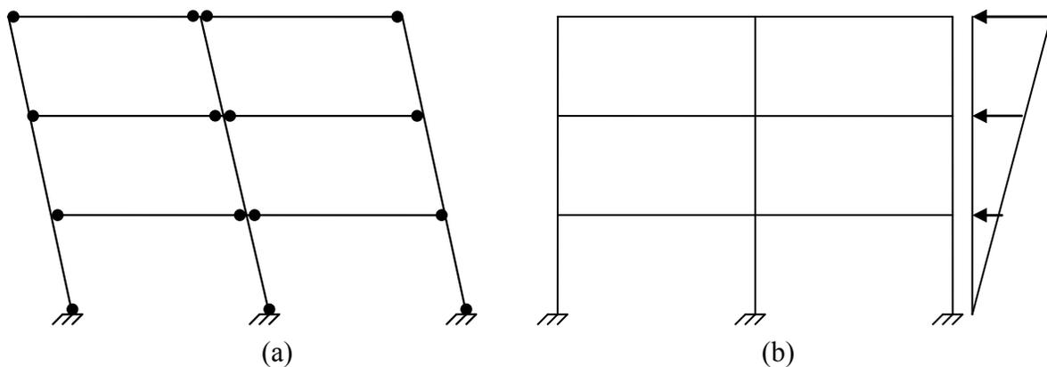
Figure 11. Assumed failure mechanism (a) and loading (b) for limit state analysis
