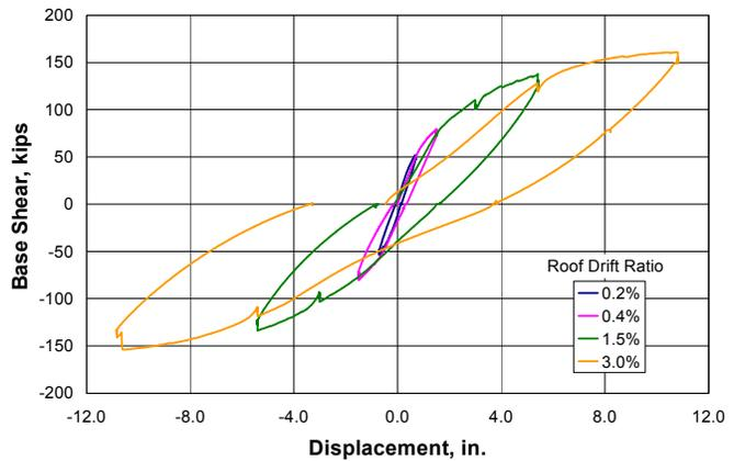
Figure 5. Base shear vs. roof displacement
