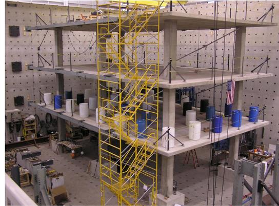
Figure 4. Completed specimen with load frames and water barrel loading.
