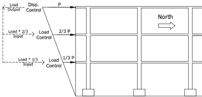
Figure 3. Load distribution and control schematic
