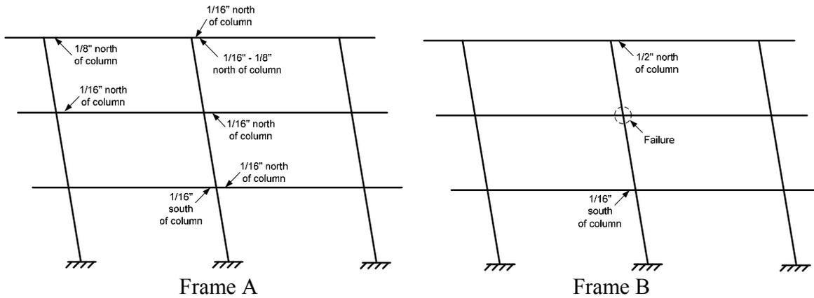
Figure 9. Vertical slab separations in south loading of Cycle 4.
