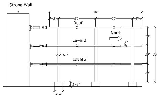
Figure 2. Specimen elevation view.
