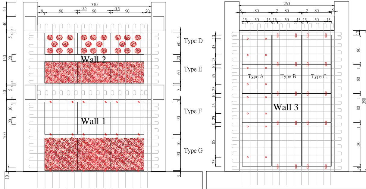
Figure 4. Layout of Exterior and Interior Veneers (unit: cm)
