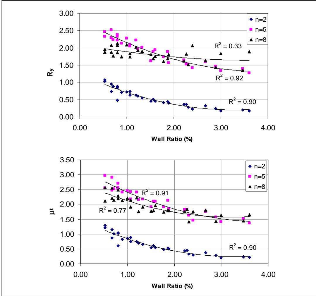
Figure 4. Variation of Yield strength reduction and displacement ductility with Wall Ratio
