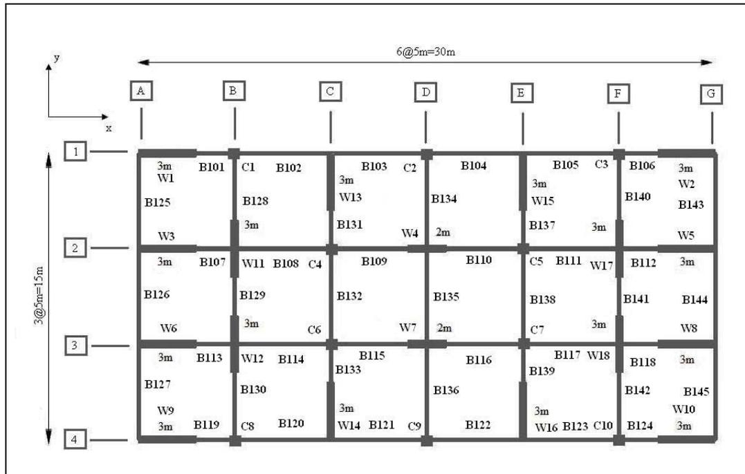
Figure 1. A typical floor plan for building models employed.
