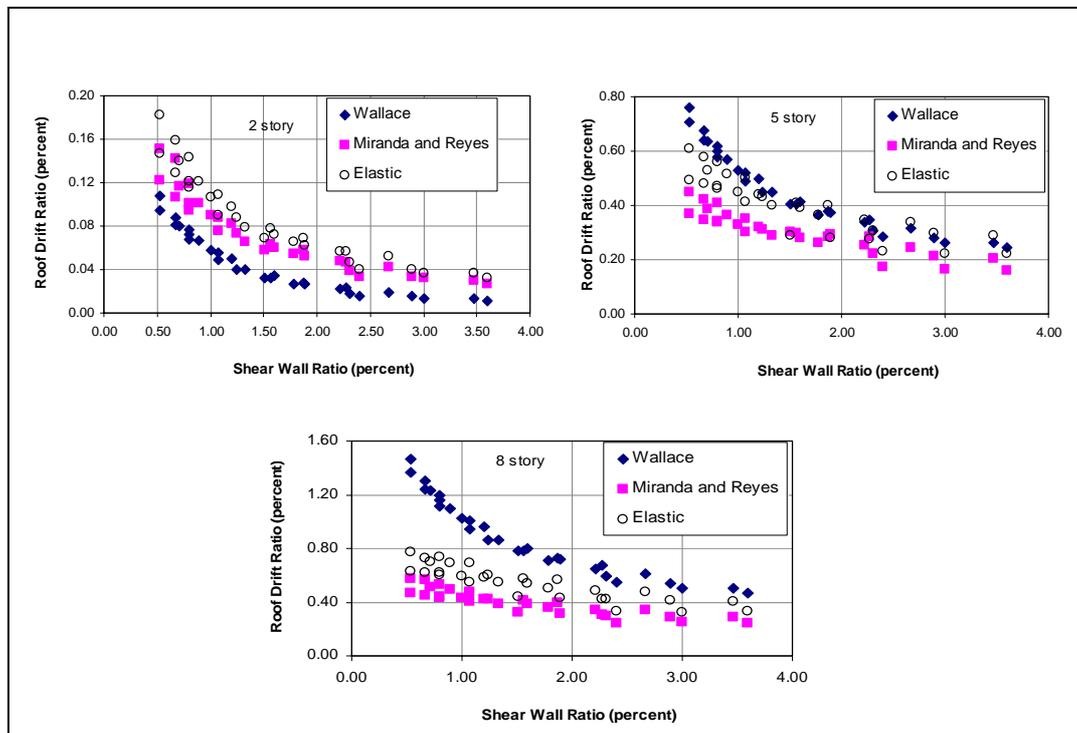
Figure 5. Comparison of Elastic Drift Ratios
