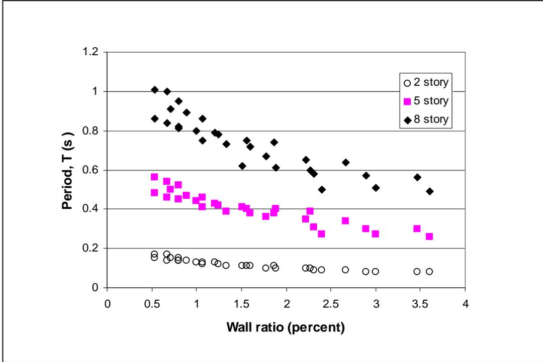
Figure 3. Variation of Period with Shear Wall Ratio.
