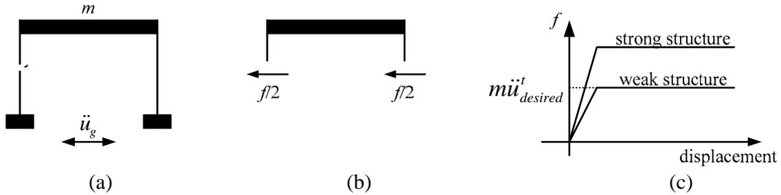
Figure 1. SDOF frame: a) description, b) free body diagram of the mass, and c) strength reduction effect.
