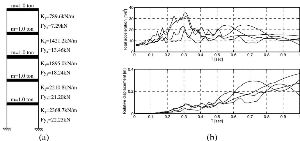
Figure 2. a) Five story shear frame, and b) response spectral values of the ground motions.
