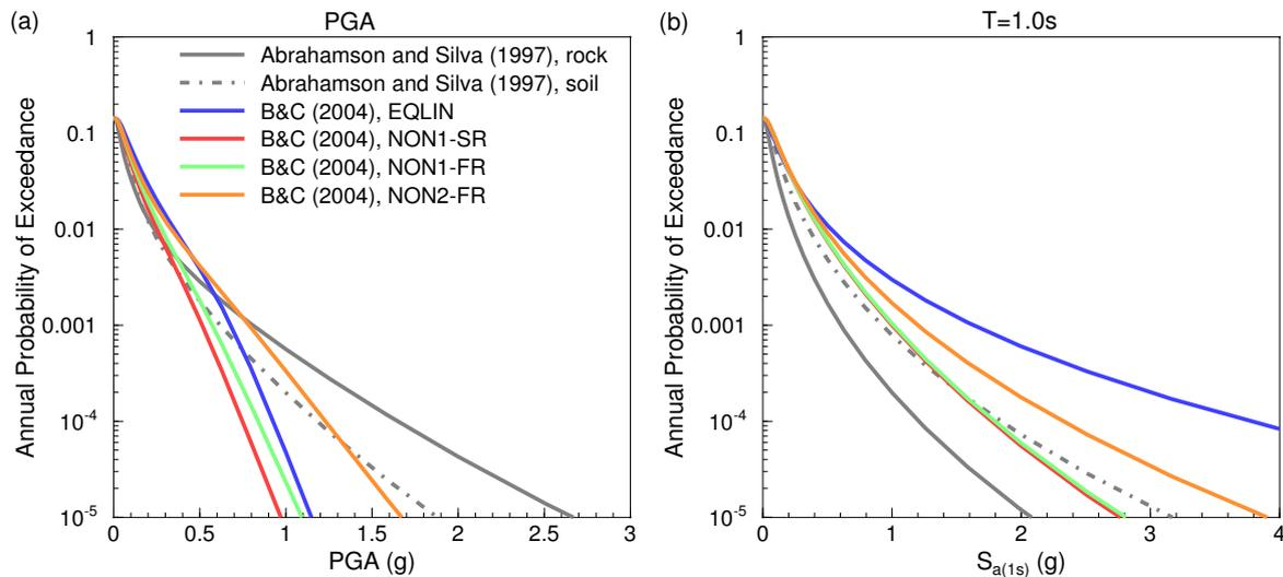
Figure 6. Hazard curves for Sylmar County Hospital for PGA and 1.0s spectral acceleration.
