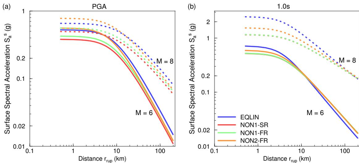
Figure 5. Modified Abrahamson and Silva (1997) equations using the Bazzurro and Cornell (2004) formulation shown for PGA and  $T=1.0s$  and two magnitude levels.
