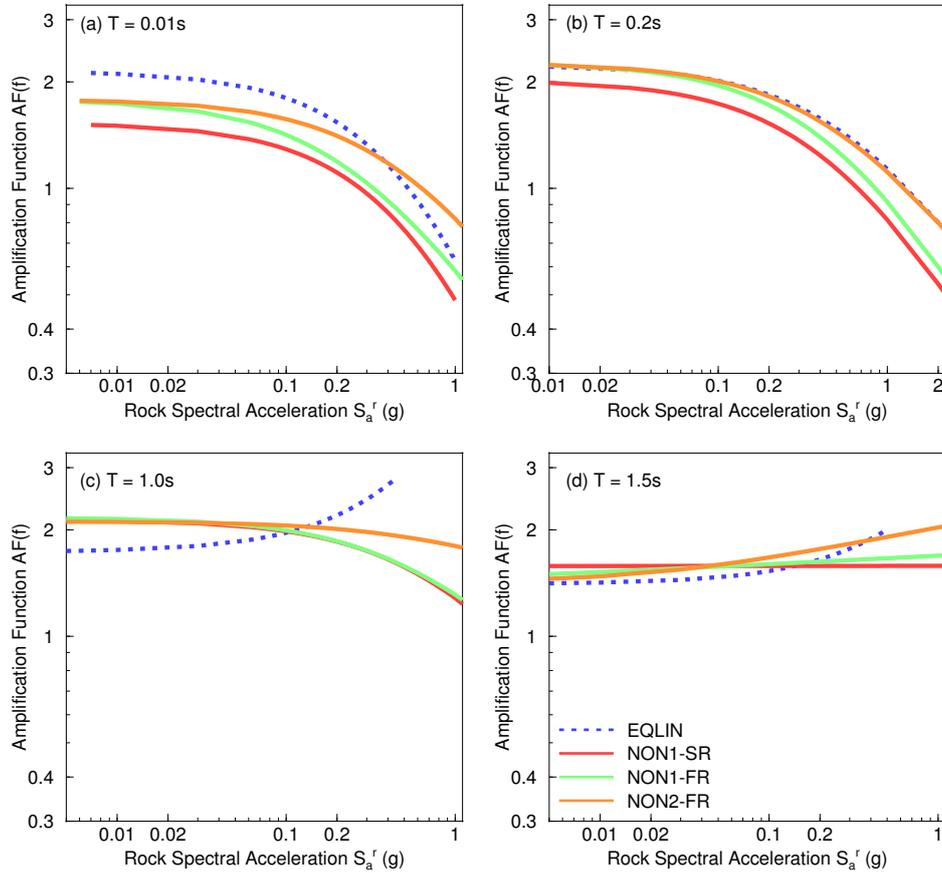
Figure 4. Mean amplification functions  $AF(f)$  for site SCH for a number of spectral periods.
