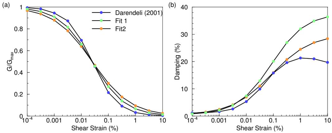
Figure 2. Different choices in fitting the modulus reduction and damping curves used in the analysis against the Darendeli (2001) curves.
