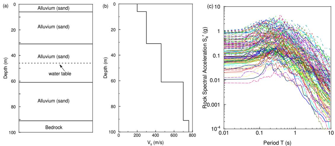
Figure 1. Site stratigraphy, shear-wave velocity profile and acceleration response spectra of the 120 rock records used in the ground response analysis.
