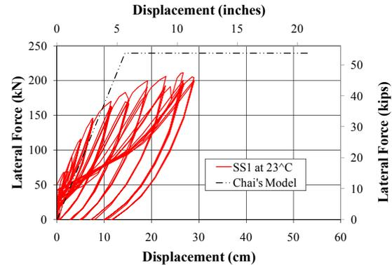
Figure 3. Global comparison of Chai's model with full-scale testing by Suleiman et al. (2006)
