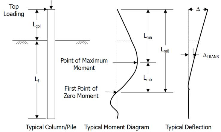
Figure 5. Definition of different variables used in the proposed new model
