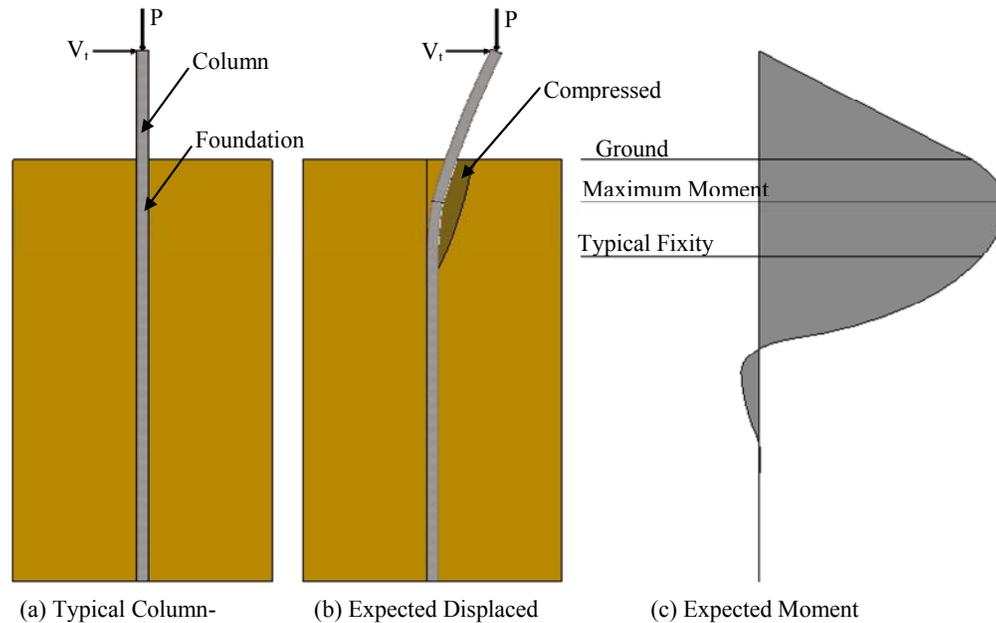
Figure 1. Expected lateral response of a bridge column supported on a CIDH shaft
