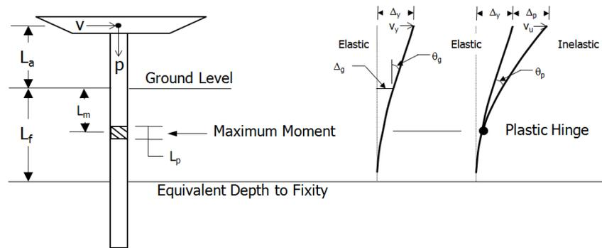
Figure 2. Equivalent fixed-base cantilever (from Chai 2002)
