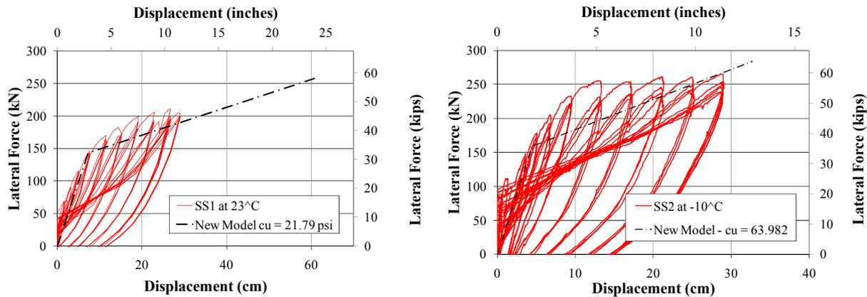
Figure 6. Verification of the proposed method with full-scale test results (a) warm weather conditions, (b) cold weather conditions
