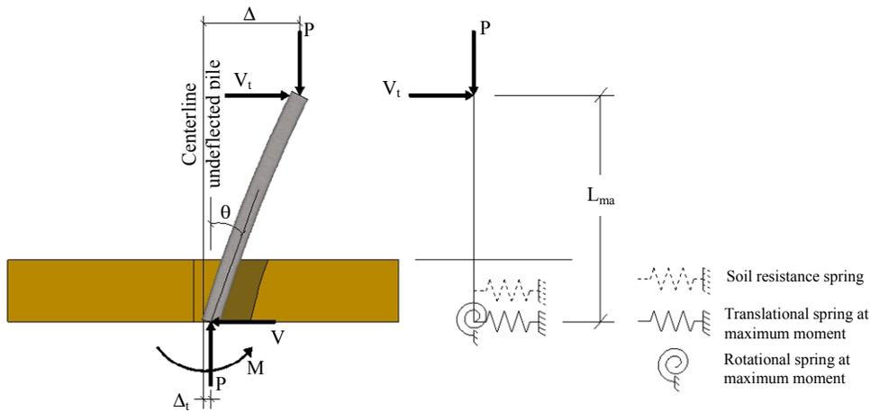
Figure 4. (a) FBD of column-foundation system; (b) proposed new approach
