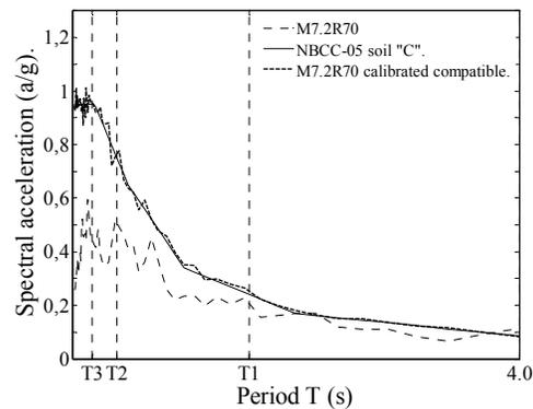
Figure 4. Response spectra of seismic signal (Atkinson and Beresnev, 1998), calibrated to be compatible to NBCC-05 design code spectra: **a)** Montreal; **b)** Vancouver.
