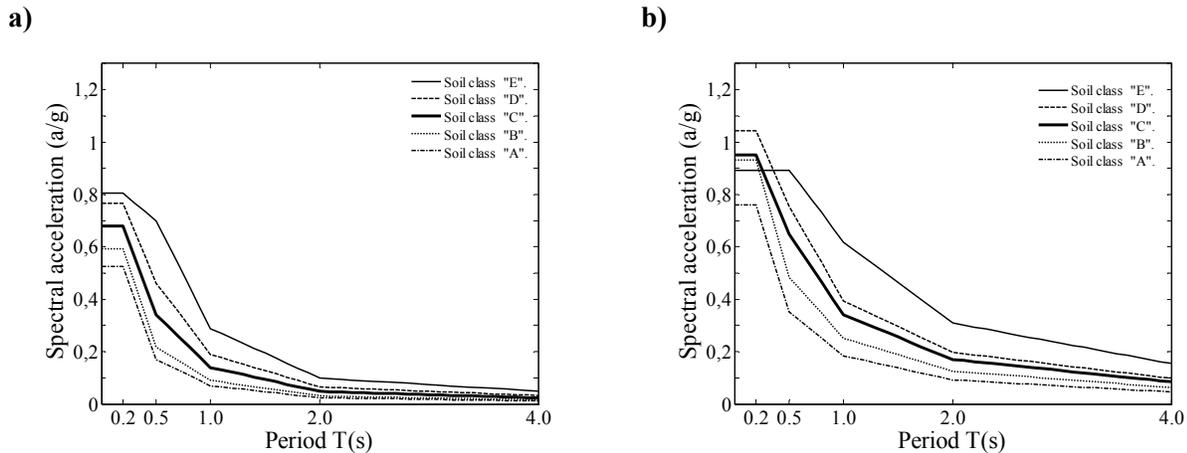
Figure 2. Design spectra for soil classes A, B, C, D, and E: **a)** Montreal; **b)** Vancouver.
