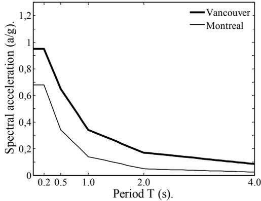
Figure 1. Uniform hazard spectrum.
