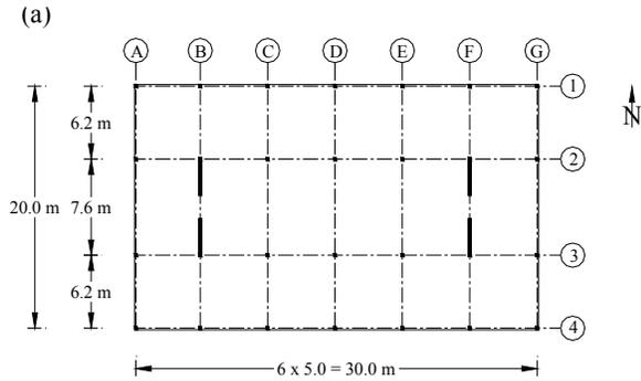
Figure 5. Plan view of coupled shear walls.
