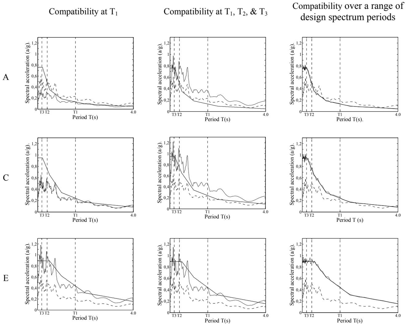
Figure 6. Spectrum compatibility for design soil classes A, C, and E: a) Vancouver design spectrum; b) M7.2R70 seismic design spectrum; c) M7.2R70 calibrated to be compatible with the design spectrum.
