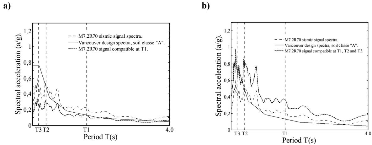
Figure 3. Spectral adjustment by vertical shift: a) at the fundamental mode period; b) at a higher mode period.
