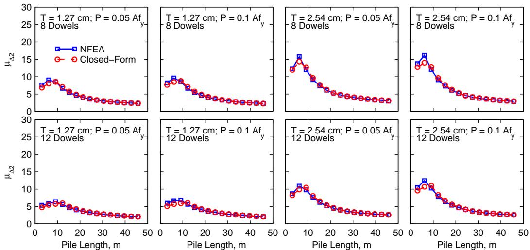
Figure 5. Displacement ductility capacity of hollow-steel pile with concrete-plug connection for design Level 2.
