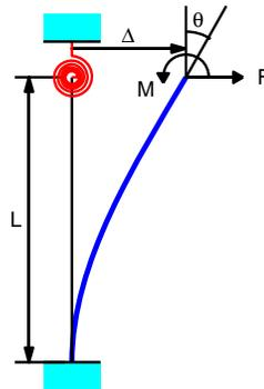
Figure 2. Simplified model of the pile with partial-moment-connection to the deck.
