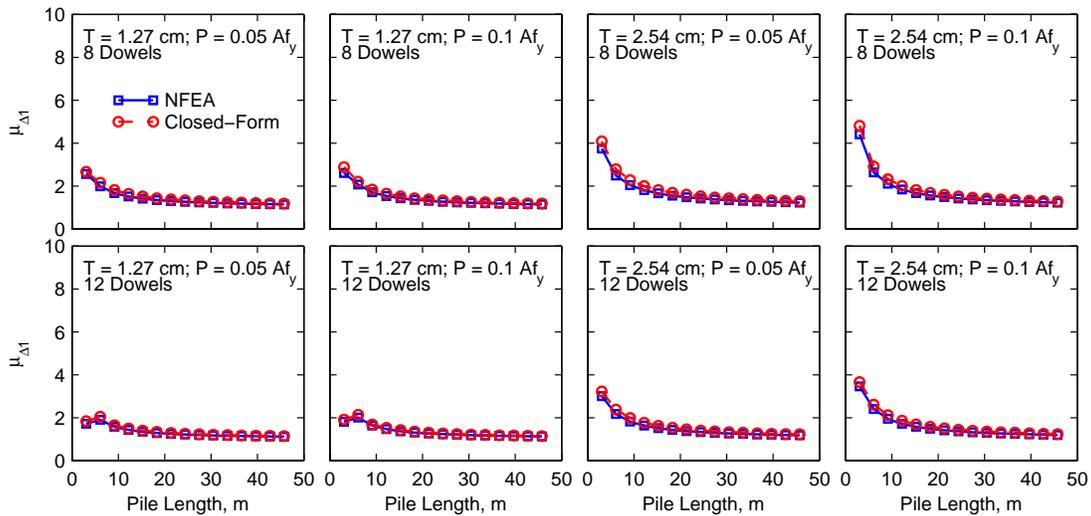
Figure 4. Displacement ductility capacity of hollow-steel pile with concrete-plug connection for design Level 1.
