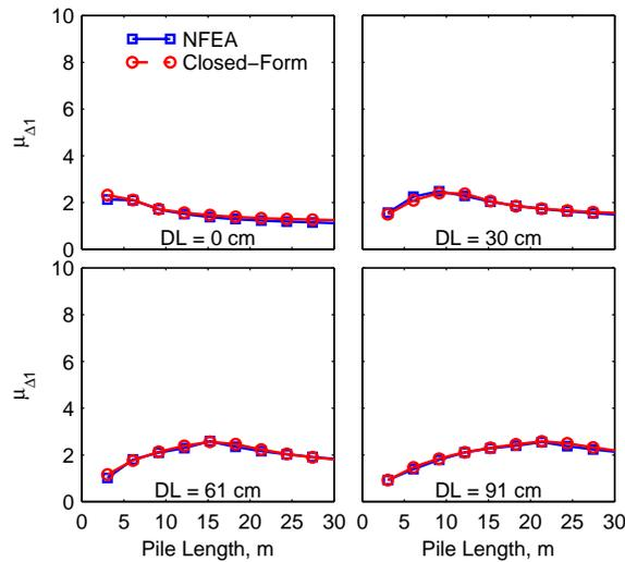
Figure 6. Displacement ductility capacity of pre-stressed-concrete pile with dowel connection for design Level 1.
