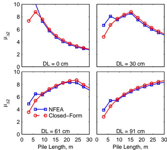
Figure 7. Displacement ductility capacity of pre-stressed-concrete pile with dowel connection for design Level 2.
