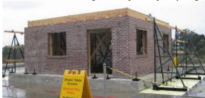
Figure 3. Test Setup and Reference Frames for Displacement Transducers
