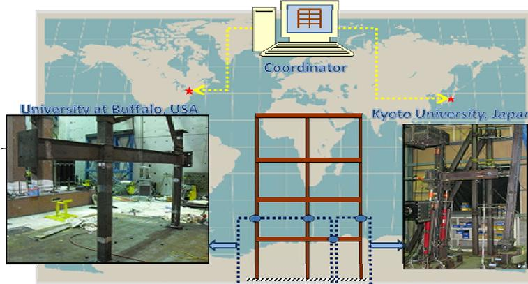
Figure 5. Illustration of geographically distributed hybrid simulation.
