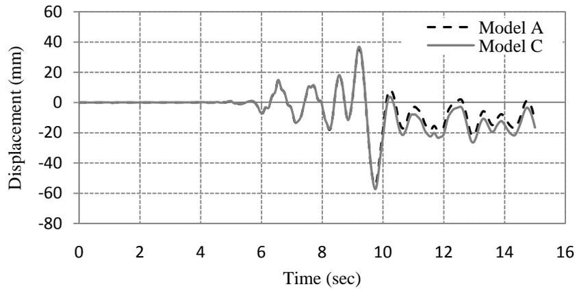
Figure 3. First story global displacement response.
