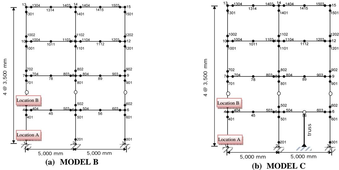
Figure 2. Models with hinges examined for substructuring.
