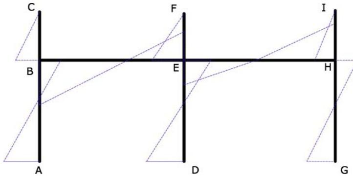
Figure 7. Moment at diagrams for hybrid test at peak displacement.
