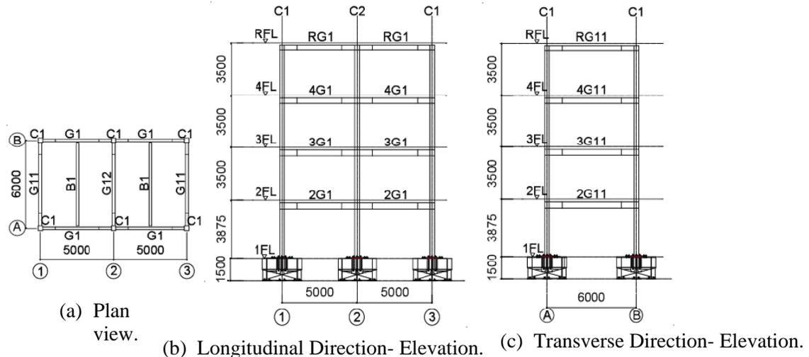
Figure 1. E-Defense Test Specimen Layout and Framing.
